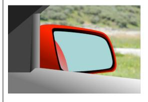
It's impossible to completely do away with blind spots but you can reduce them a great deal by the proper Now, sitting upright, with both outside mirrors adjusted this way, as a vehicle moves over to pass, you'll see it divided between the two mirrors. Once it moves completely into the other lane, you'll be able to see it in your outside mirror almost up to the point where it enters your peripheral (side) vision.
