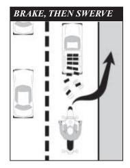
A swerve is any sudden change in direction. It can be two quick turns, or a rapid shift to the side. Apply a small amount of hand pressure to the handlegrip located on the side of your intended direction of escape. This will cause the motorcycle to lean quickly. The sharper the turn(s), the more the motorcycle must lean.
